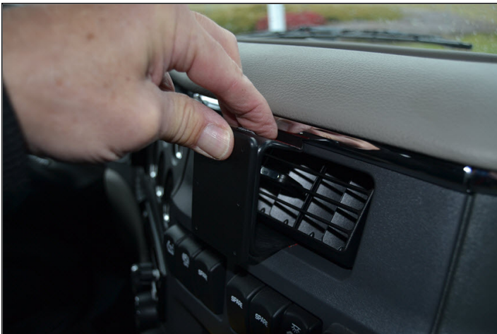
3. Flex the top angled edge of the ProClip into the seam between the dash panel and inside of the top of the vent.
