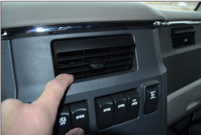
1. Tilt the vent downward to find the seam between the dash panel and inside of the vent.
