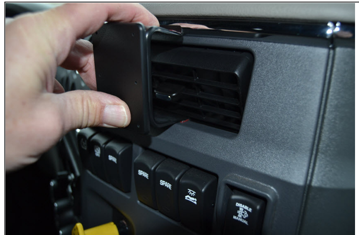
2. Place the ProClip in your hand so the ProClip label (sticker) is in an upright position, or if vertically positioned; the P in ProClip is at the top. Insert the lower angled edge of the ProClip into the seam between the dash panel and inside of the bottom of the vent.
